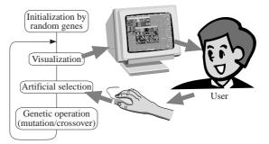
Figure1: Schematic diagram of SBART.
